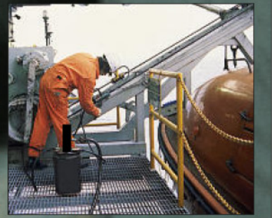
The Masto Lubricator is portable, but it can also be mounted permanently, for example by installing a lubricating chamber on each lifeboat rope with a T-coupling.
