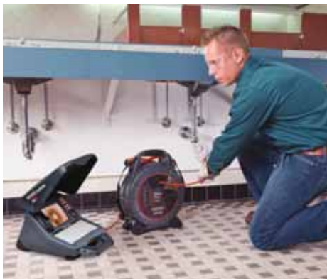
SeeSnake nanoReel with micro CA-350 used as a monitor and recording device. See page 13.24 for details on the CA-350.
