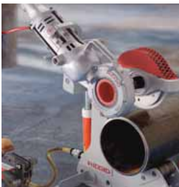
Model 258 Pipe Cutter with No. 700 Power Drive in use for cutting
